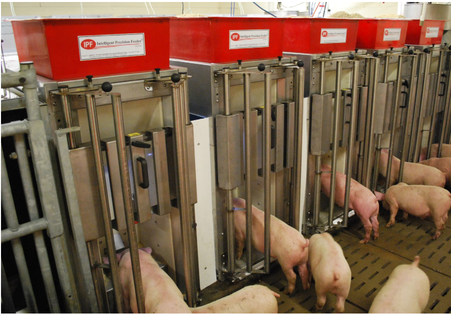
Figure 4. Individual feeders allow one pig at a time to request feed. Each animal is identified by the plastic button ear tags containing passive transponders, which provide pigs with diets that are tailored daily to individual requirements of each pig.
